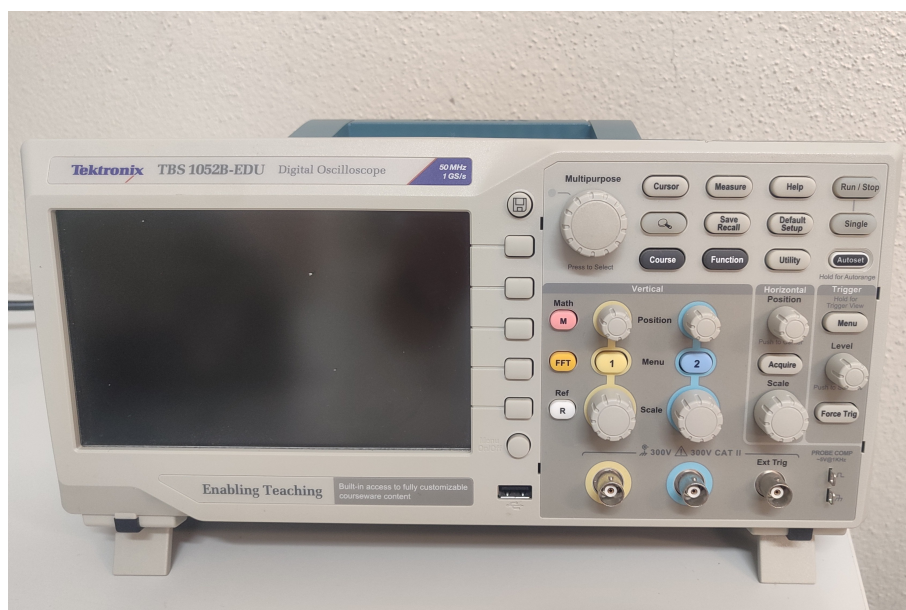
Figure 3.2: Tektronix TBS 1052B-EDU digital oscilloscope used for signal validation and communication analysis.
