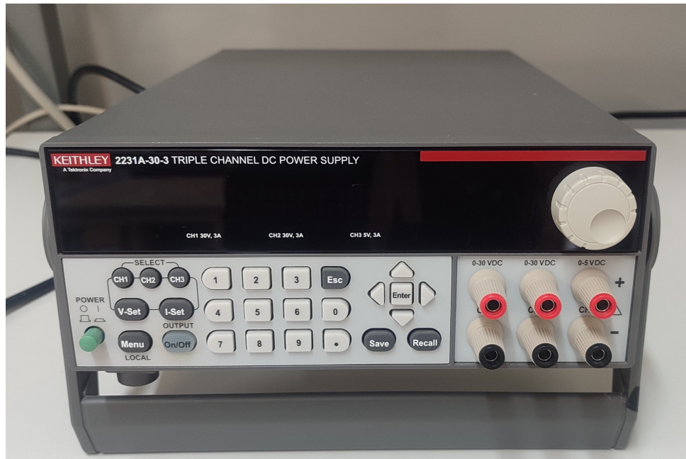
Figure 3.1: Keithley 2231A-30-3 benchtop power supply used to energize the system during experimental tests.
