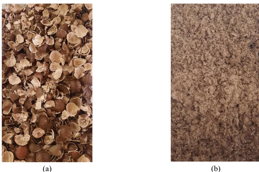
Figure 4. (a) Chestnut shells after peeling; (b) ground chestnut shells.
