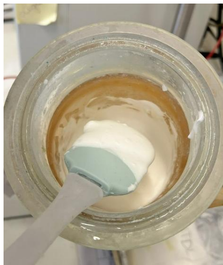
Figure A1 – Visual appearance of the DTX274_2 dispersion showing phase destabilization and gel formation after synthesis.
