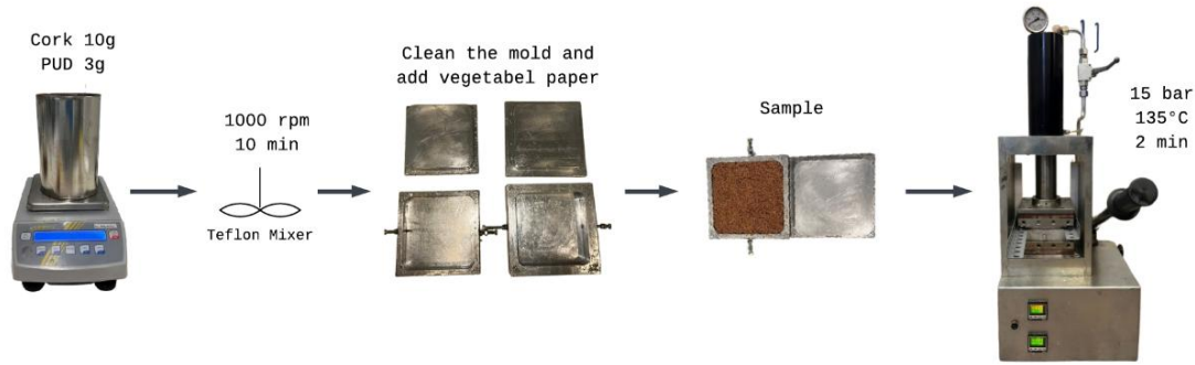
Figure 4 – Representation of the manufacturing process of cork-based composites using aqueous polyurethane dispersions
